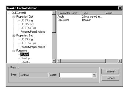
All the methods and properties listed in this dialog can be directly sent to the object representing the OCX control. The class for a simple data window containing a Light Lib OCX is shown below:
