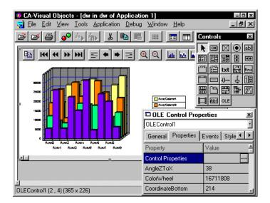
When the Window Editor is invoked, the Visual Objects IDE View menu extends to include "Test Mode...", thus giving the Window Editor two modes or states, design mode and run (or test) mode. OLE controls will not be *active* at design time (they will not have a window handle yet), but will appear only as a representation of contents. This is done in order to increase performance and memory by minimizing the number of open windows. When in test mode, however, the controls will be activated.
