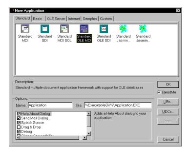
This creates the Standard OLE Menus module, which contains the EmptyShellMenu and StandardShellMenu entities. StandardShellMenu contains OLE menu items such as Insert Object, Paste Special, and Links.
