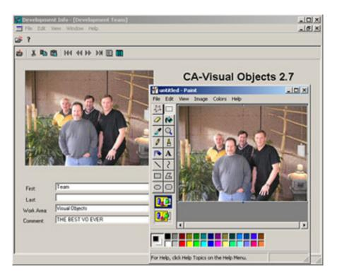
Notice that Microsoft Paint runs in a separate window, and that the OLE object inside the Visual Objects container is grayed out as long as the object is being edited. To close Microsoft Paint during the out-of-place activation, click anywhere on the Visual Objects form.
